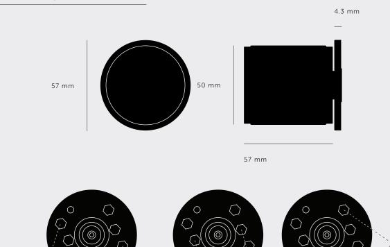
A pair of unsprung solid metal door knobs, with an architectural 4 mm thick rose.
